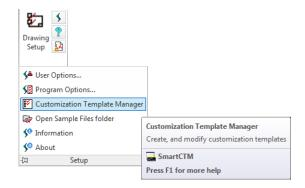
In the Customization Template Manager dialog, either select the Default (original SmartDraft layers), or NCS (our version of the National CAD standard layers) customization template as the template to use as the base of your own company's SmartDraft Customization Template.
