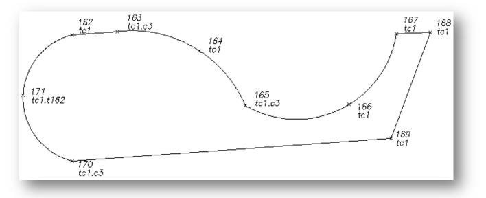
**Note:** Field crews do not have to add a description suffix at a point of reverse or compound curve, since the .C3 suffix code only reads the (3) consecutive points. Field crews can add a new C3 to start a new 3-Point Curve. PConnect checks for direction changes between segments and automatically determines the presence of a PRC or PCC, so there is no need to identify the PRC or PCC when using the C3 suffix code. See points162 - 171 above.
