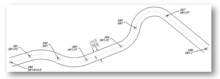
Note: The offset polylines will create a fillet with a zero (0) distance if the offset is larger than a calculated curve radius.
