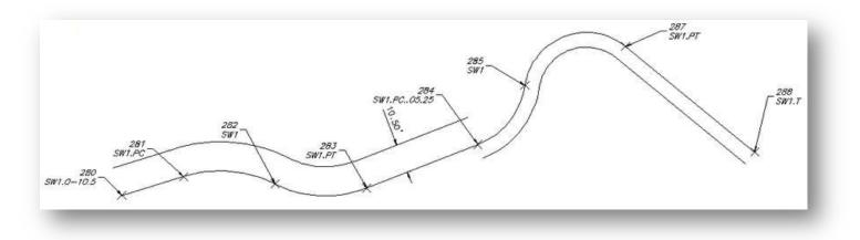
**Note:** There is not a transition from the first Offset code offset distance (-10.5) to the second Offset code offset distance (5.25); the first one stops, and the second one begins.
