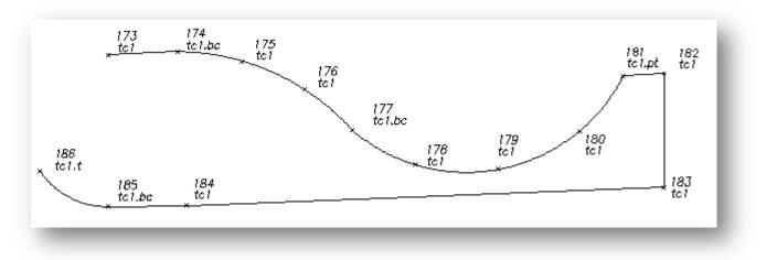
**Note:** If only two points are encountered after the Best Fit Curve (.BC) code, and the bearings created between the first two points and the second two points differ by less than five (5) degrees, the Begin Curve (.PC) calculation method is used to create a reverse curve. If the Best Fit Curve method was used, the curved segments would appear almost like two straight segments.
