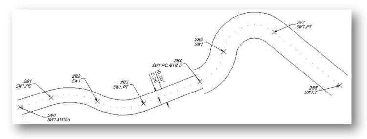
**Note:** There is not a transition from the first Middle code offset distance (10.5) to the second Middle code offset distance (18.5); the first one stops, and the second one begins.
