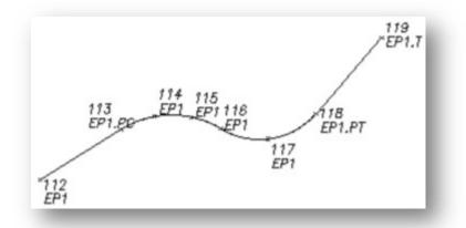
**Note:** Field crews do not have to add a description suffix at a point of reverse or compound curve. As long as there is not a straight segment, do not add the End Curve (.PT) code, and the command will draw the reverse or compound curve segments. PConnect checks for direction changes between segments and automatically determines the presence of a PRC or PCC, therefore, there is no need to identify the PRC or PCC with a PT/PC.
