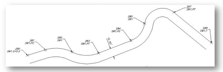
Note: The offset polylines will create a fillet with a zero (0) distance if the offset is larger than a calculated curve radius.
