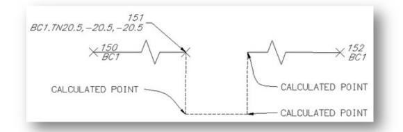
**Note:** The code assumes the previous segment was a straight segment, and this suffix code is ignored if in the middle of any of the curve suffix codes. This code can be combined with a termination code (.T, .CS, or .CC).
